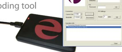
Idesco EPC Writer is an elegant and compact-size tool for encoding EPC Class 1 Generation 2 trasnsponders mainly in office environment. It consist of an Idesco EPC Writer Application and a Desktop read/write device equipped with USB interface.
